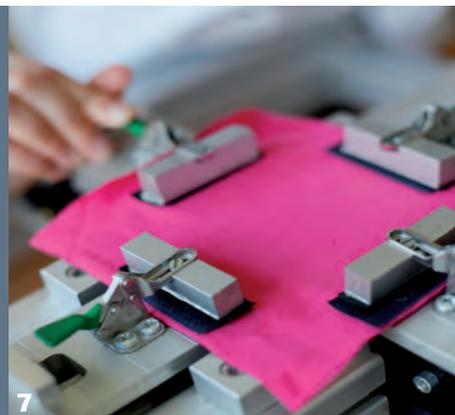
7 Before measuring the textile is stretched in a specified manner with the aid of a stretching device.
